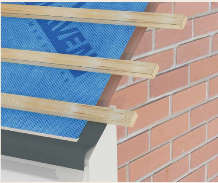
felt & batten in the usual way
